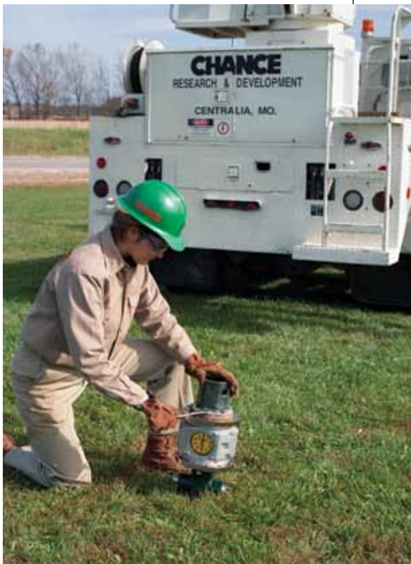
5 1/4" Bolt Circle on Standard-Strength Tooling (10,000 ft. lb.)
