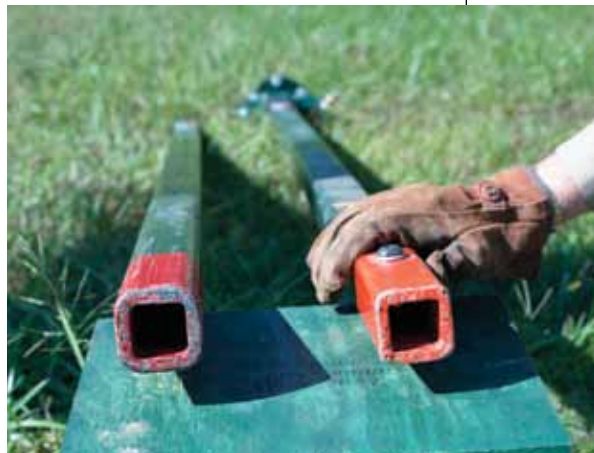
Note the difference in size of the 15,000 ft.-lb. wrench tube on the left compared to the 10,000 ft.-lb. standard tube on the right.
