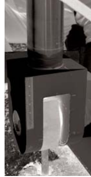
Using a transit, anchor creep is monitored as load is applied to the installed anchor.
